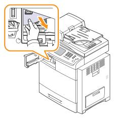
4 Pull up on the stacker lever and then close the stacker front cover.
